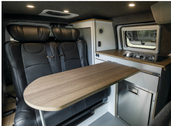
Fold Down Table: Made of 11-ply baltic birch, the table is easy to set up and is conveniently stored on the galley
